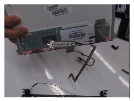
The screen is fully disconnected from the screen bezel and can now be removed.
