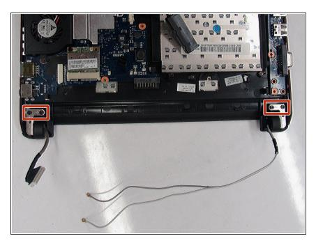
Use a Phillips #00 screwdriver to unscrew the four 5 mm screws located on the two hinges.
