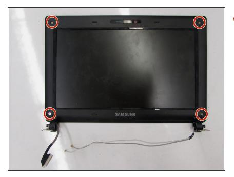
Use a Phillips #00 to unscrew the four 5mm screws located at the top and bottom corners of the screen bezel.
