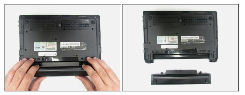
• While holding the left and right hand switches in the "unlocked" position, push the battery away from the computer.
