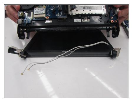
Slowly remove the screen case from the rest of the laptop by pulling the screen case out of the hinge sockets.
