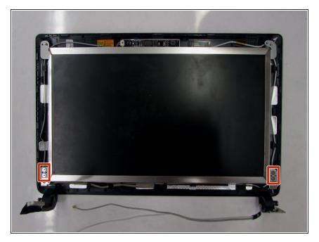
Use a Phillips #00 screwdriver to unscrew the four 5mm mounting screws that secure the screen to the bottom case.
