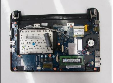
The computer should be open with the motherboard exposed and internal components exposed. You should now be able to access the Fan and RAM. There are more necessary steps to follow before accessing the screen and keyboard.
