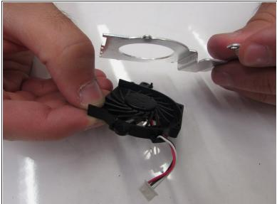
Remove the fan from the metal CPU housing.
