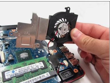
Use the phillips #00 screwdriver, to unscrew the two 5mm mounting screws labeled 1 & 2 on the right and left hand side of the metal casing labeled CPU.
