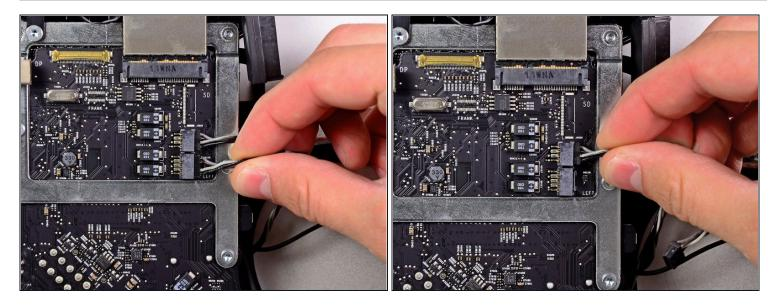
• Disconnect the left speaker and right speaker cables by pulling their connectors toward the right side of the iMac.
