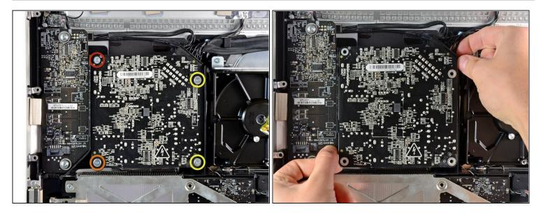
A Be careful not to touch any solder joints on the back of the power supply. Capacitors may be charged enough to give you a dangerous shock.
