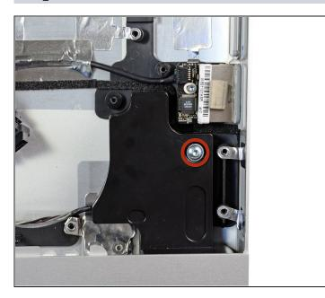
• Remove the single 13 mm T10 Torx screw securing the right speaker to the outer case.
