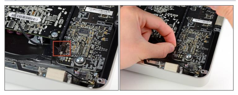
• Pull the vertical sync cable connector out of its socket on the LED driver board near the top left corner of your iMac.
