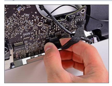
• Disconnect the audio port cable by pulling its connector away from the front face of the logic board.
