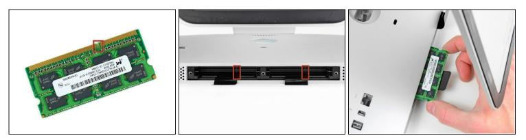
A When installing new RAM modules, it is important to orient them correctly.
