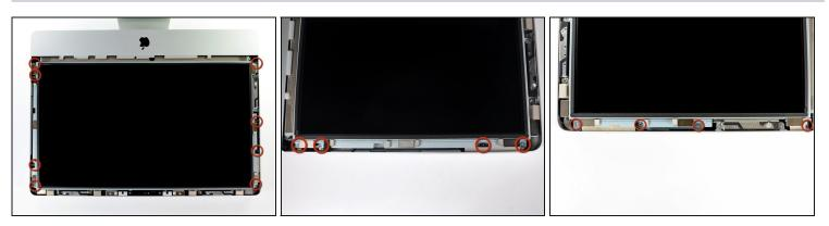
Remove the eight 8 mm T10 Torx screws securing the display to the outer case.
