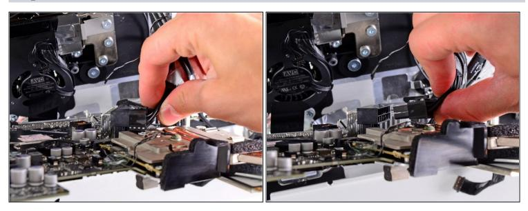
• Depress the locking mechanism and carefully pull the DC-In cable out of its socket on the back of the logic board.
