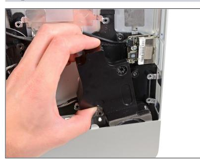
• Pull the right speaker away from the right side of the outer case and lift it out of the bottom edge of the iMac.
