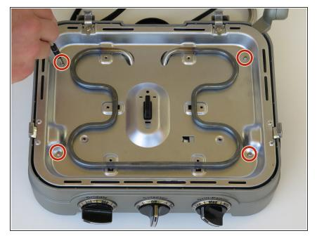
Remove the four 30 mm Phillips #2 screws that secure the bottom heating apparatus.
