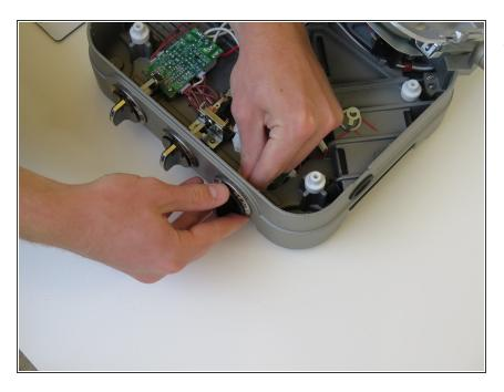
Pop the new knob back into the hole and the repair is complete.
