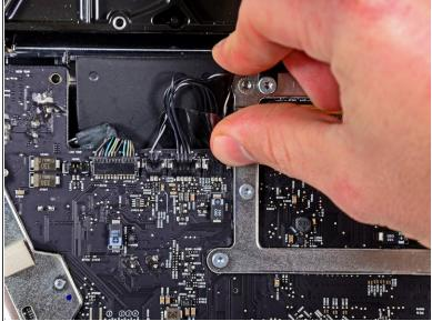
Pull the optical drive thermal sensor connector toward the top edge of the iMac to disconnect it from its socket on the logic board.
