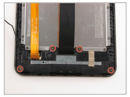
Remove the four 3 mm Phillips #000 screws securing the speaker assembly.
