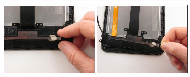
Remove the speaker assembly from the device.
