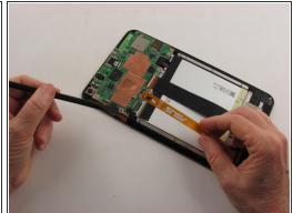
Use the flat end of the nylon spudger to flip up the retaining flap of the Zero Insertion Force (ZIF)
