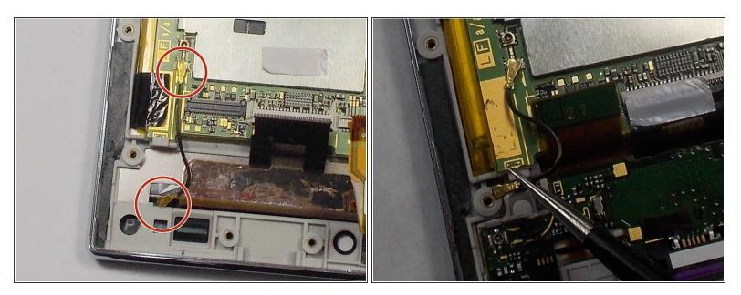
Remove the wire from the two marked connections using tweezers to pull the wire apart from the device.
