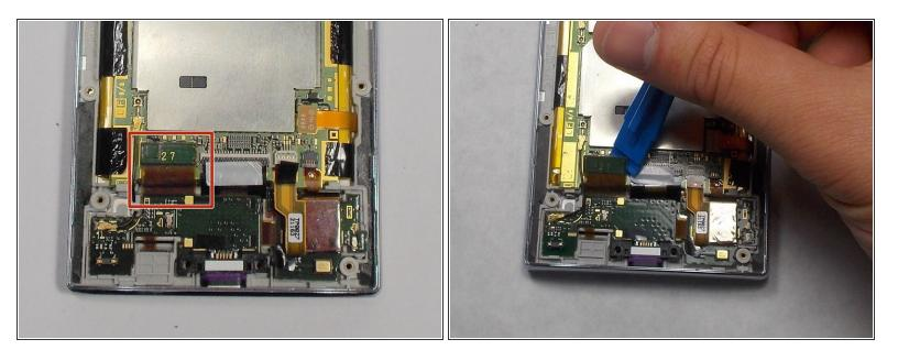
Disconnect the wire by lifting it up with a plastic opening tool.
