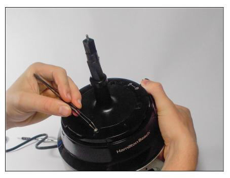
Remove any excess glue that is adhered to the screws with the precision <u>tweezers</u>.
