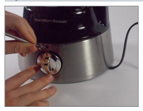
Using a metal spudger, pry the switch from the front of the device.
