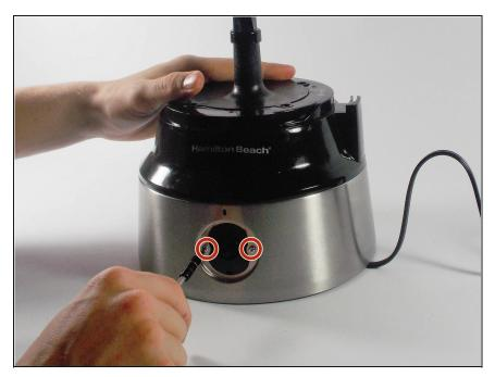
• Remove the two 4 mm screws underneath the on/off switch with a JIS #1 screwdriver.
