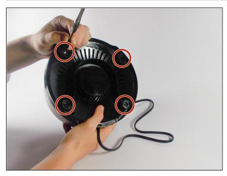
Using a JIS #1 screwdriver, remove each of the four suction cups that are attached to the bottom of the food processor.
