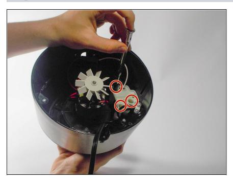
Using a JIS # 1 screwdriver, remove the three screws on the white bracket.
