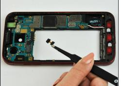
Remove the camera from the plug at the top of the phone with tweezers. It should pop out fairly easily.
