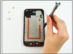
Remove the screws around the plate
