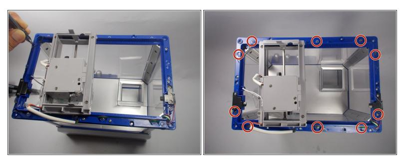
• Remove the ten 6 mm phillips #1 screws from the top flange.
