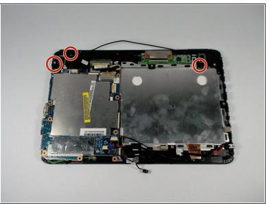
After removing the battery use a Phillips head #00 screwdriver to remove the 3.0 mm screws holding the dual speakers in place.
