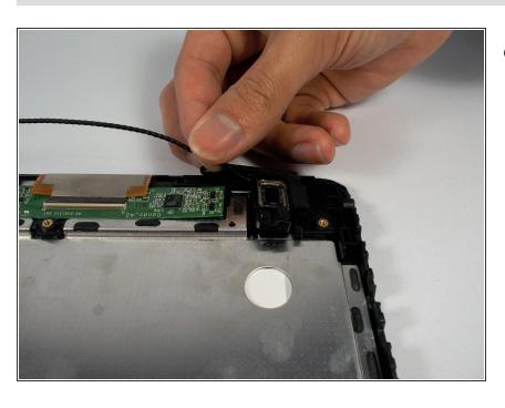
Once the screws are removed, lift up on the speakers to remove them from the case.
