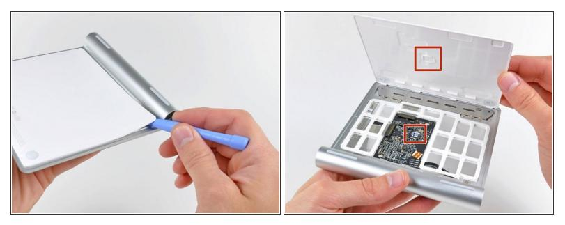
Use a plastic opening tool to separate the adhesive securing the back panel's left, right, and top edges.
