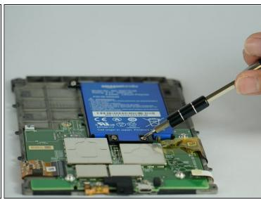
Unscrew the three 3.0 mm Phillips #000 screws that are securing the battery.
