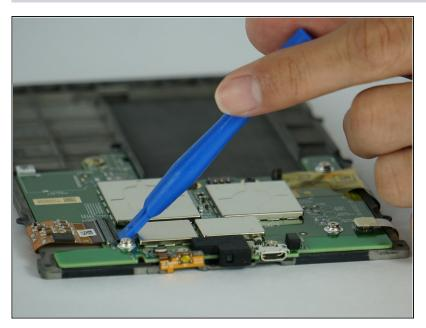
Flip the black latch with a plastic opening tool, and then gently pull back the orange ribbon cable.
