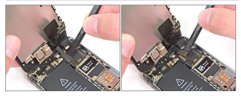
• Finally, disconnect the digitizer cable connector.
