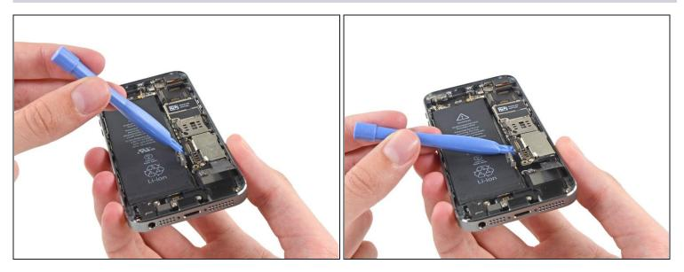
• Use a plastic opening tool to lift the logic board up enough to grab with your fingers.
