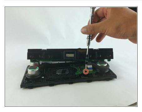
Remove the 12.5 mm screw mounting the motherboard using a Philips #2 screwdriver.
