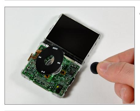
Gently turn the iPod over to the other side. The click wheel button can now be removed from the rest of the iPod.
