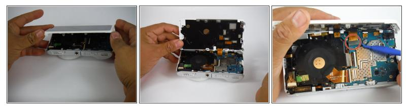
With the screen freed, gently lay the camera on its face, so that the battery compartment faces up.
