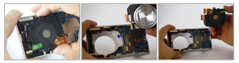
Now that the screws and ribbon cables have been removed, gently pull the lens assembly up from the the camera and remove it.
