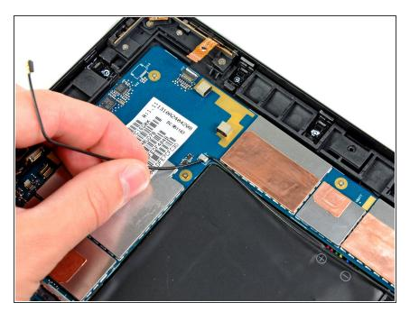
De-route the lower antenna cable along the top edge of the battery and carefully pull it out from under its retaining clip near the top right corner of the battery.
