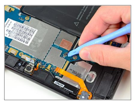
Pry up the lower antenna cable connector from its socket on the motherboard.
