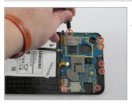
Remove the seven 4mm Phillips J000 screws holding the motherboard in place.
