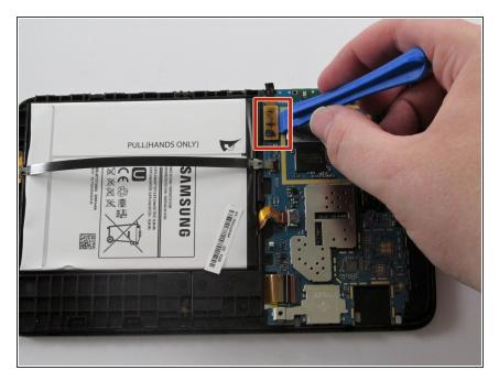
Use the plastic opening tool and gently pry up the tab holding the motherboard in place.
