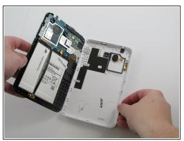
After separating the tape holding the screen and case together, slowly start taking the screen off the case from the opposite side of the side with the buttons
