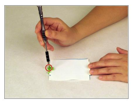
Use a Phillips screwdriver to remove the screw from the green clip that holds the two screen layers together.
