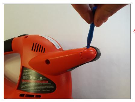
• Using the plastic tool, detach the handle tab as shown.
