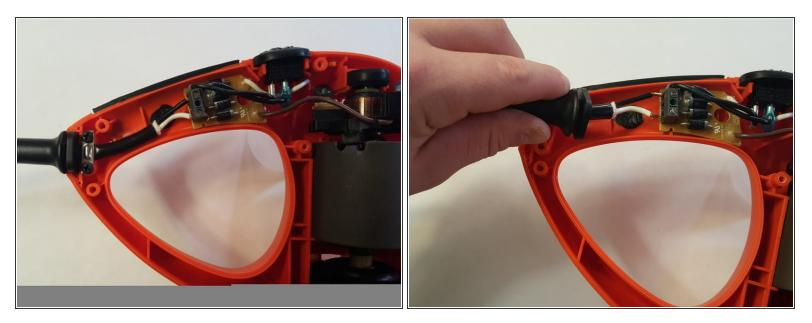
• Gently pull the power cord out from the control module.
