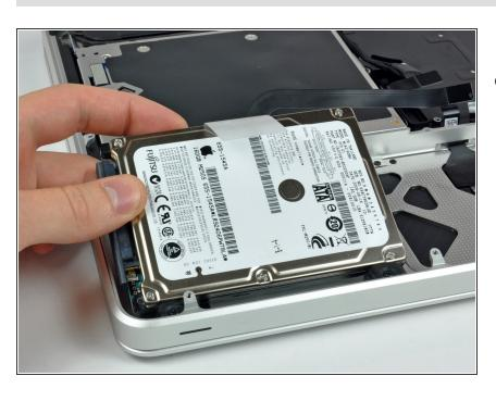
Lift the hard drive from its free edge and pull it out of the chassis, minding the cable attaching it to the computer.
