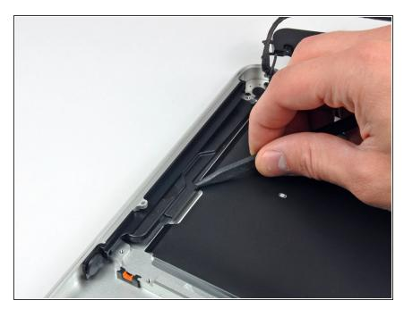
Use the tip of a spudger to pry the right speaker up off the adhesive securing it to the upper case.
