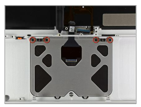
Remove the four 1.2 mm Phillips screws highlighted in red.
