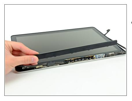
Remove the clutch cover from the display.
