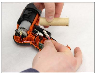
Detach the contact by pulling the contact away from the battery.
