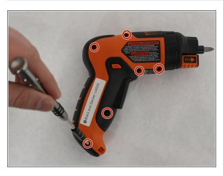
Remove all six of the 12-mm long case screws with a Philips #1 Screwdriver. These screws can be found on the side of the LI4000 with the "Warning" sticker.
