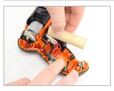
Locate the other contact on the rear side of the battery.
