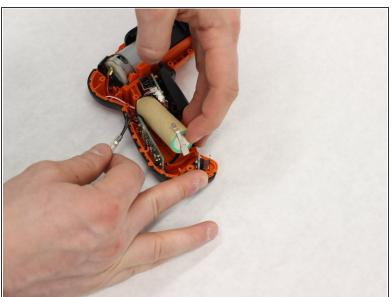
Gently lift the end of the battery out of the plastic casing
