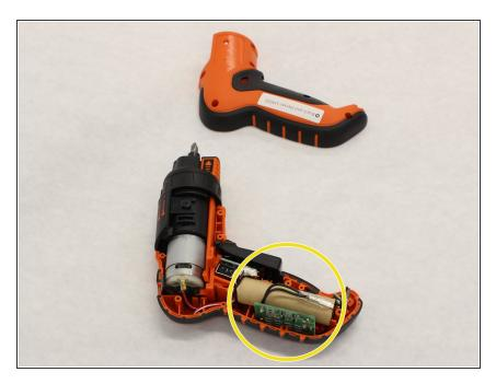
Locate the battery. The cardboard covered cylinder is the rechargeable battery.
