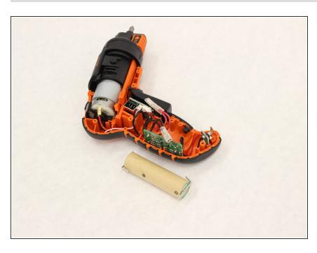
To install a new battery, repeat the steps in reverse order with a new battery.
