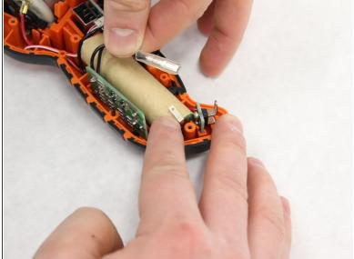
Detach the contact by pulling the contact away from the battery.
