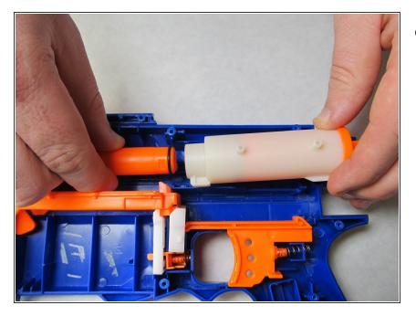
Remove white air chamber by depressing the orange trigger apparatus and pulling backwards off of the barrel.
