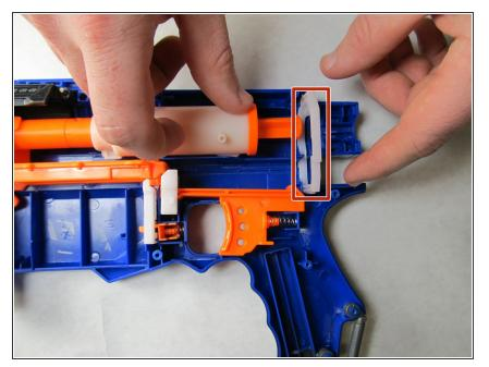
Slide the white air chamber forward and remove the white alignment bracket.
