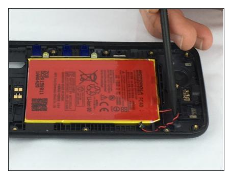
Use a spudger to carefully pull the battery wire connector out from under the bridge.
