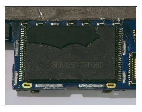
The 8GB NAND flash chip (Toshiba TH58NVG6D1DTG80), revealed after removing a soldered-down cover. This chip was covered by a plastic shield as well, which we've partially removed to see the markings beneath.
