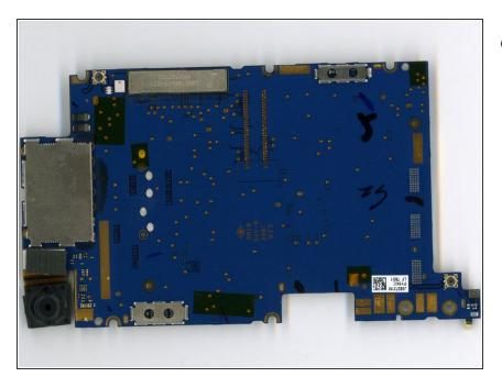
The back of the logic board, after pulling up the metallic shielding.
