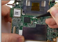
• Unhook the small plastic tooth from the underside of the motherboard. This can be accomplished with <u>tweezers</u>.
