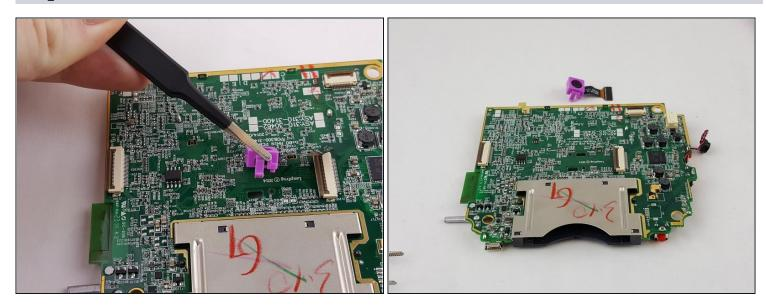
• Pull the camera out of the top of the motherboard for replacement.
