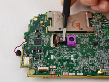
• Unplug the rear facing camera located in the top center of the motherboard.
