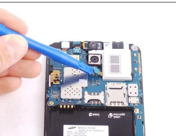
Unhook the ribbon cable clip with the plastic opening tool and remove the audio jack.
