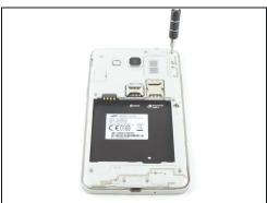
Remove the nine 4mm screws screws from the midframe with a Phillips #000 screwdriver.
