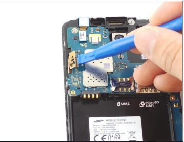
• Unhook the other ribbon cable clip to the screen with the blue plastic opening tool.
