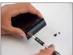
Remove the five 4.0 mm Phillips #000 screws on the back panel.
