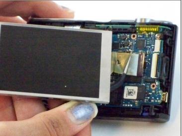
• Gently pull on the ribbon wire disconnecting from the ZIF connector (connecting the LCD screen to the motherboard) with the <u>tweezers</u>.
