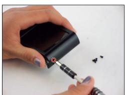
Remove the five 4.0 mm Phillips #000 screws on the back panel.
