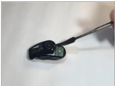
Finish the disassembly of your NikePlus Sportband by utilizing the metal spudger tool on the short edge to pry the external body pieces apart. To reassemble your device, follow these instructions in reverse order.
