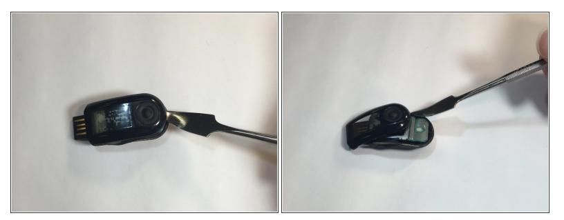
• Finish the disassembly of your NikePlus Sportband by utilizing the metal spudger tool on the short edge to pry the external body pieces apart.
