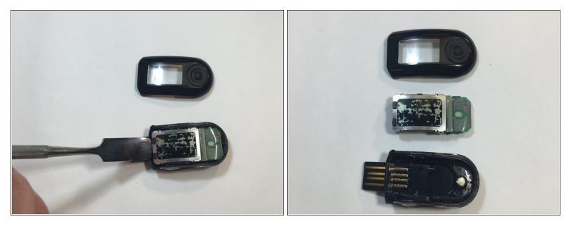
After the cover had been removed, use the metal spudger tool to remove the body of the device from the casing.
