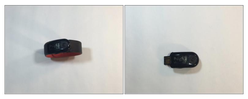
• To begin the disassembly of your NikePlus Sportband, first remove the device from the rubber wristband.
