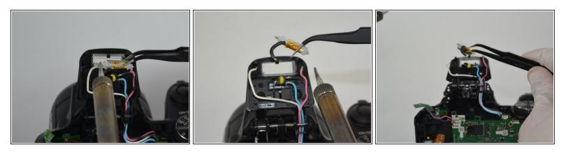
• Using the tweezers remove the flashbulb.
