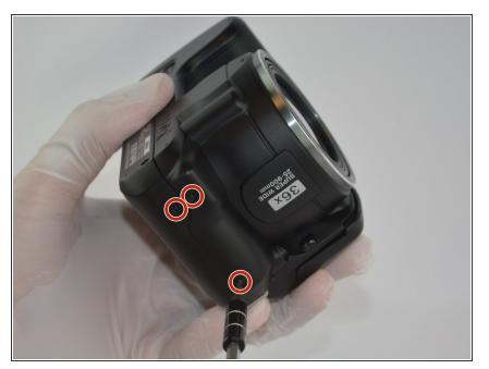
Use your Philips Head Screwdriver to remove the M3 x 4mm screws from the left side of the device as indicated by the pictures.
