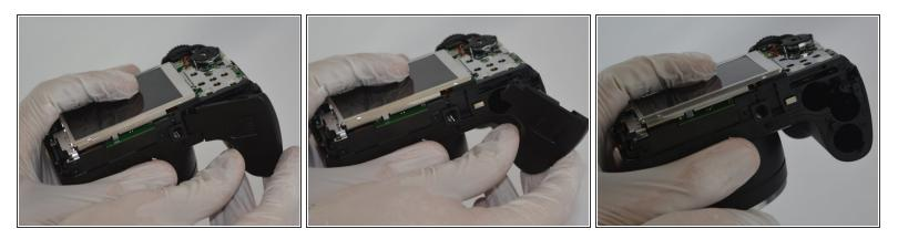
• Once the back plate is removed twist the battery cover clockwise and it should easily dislodge.
