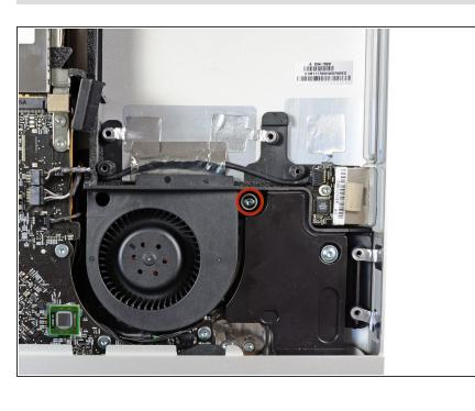
Remove the single 13 mm T10 Torx screw securing the optical drive fan to the outer case.
