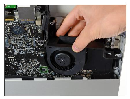
Pull the optical drive fan off the pins attached to the outer case.
