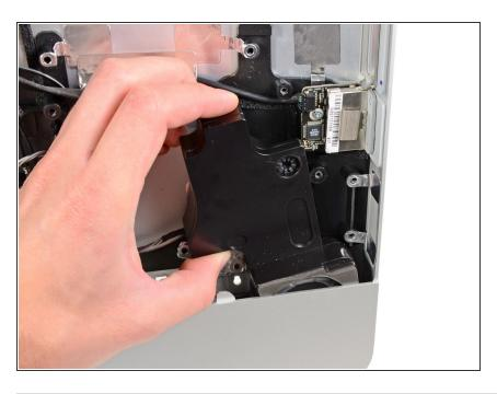
Pull the right speaker away from the right side of the outer case and lift it out of the bottom edge of the iMac.
