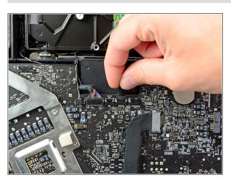
Pull the hard drive fan connector toward the top edge of the iMac to disconnect it from its socket on the logic board.
