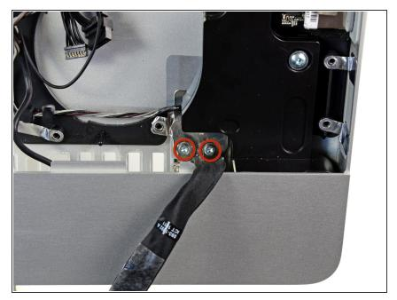
Remove the two 5 mm T10 Torx screws securing the audio ports to the outer case.
