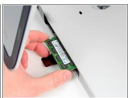
Repeat the process in the previous steps to remove the RAM module(s) from the other side of the RAM bay.
