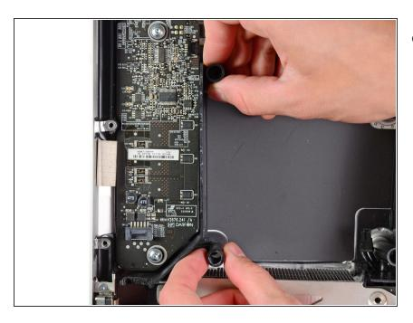
Remove the plastic wall that is installed directly to the right of the LED driver board.
