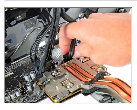
Being careful not to damage the socket on the logic board, gently pull the hard drive SATA data cable straight out of its socket on the logic board.
