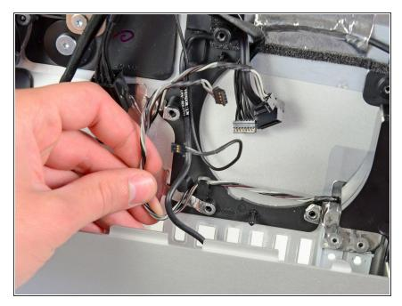
De-route the right speaker cables from the black plastic clips attached to the outer case.
