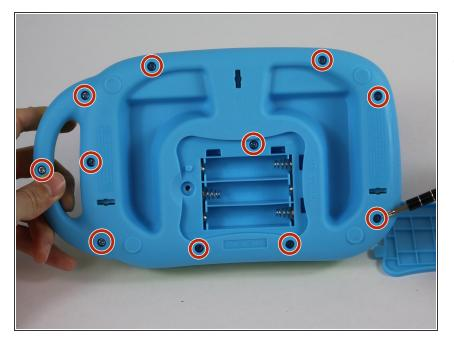
Remove the eleven 10mm screws from the back of the device with a a PH1 phillips head screwdriver.
