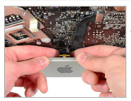
Use your fingers to lift IR sensor assembly straight up and out of the outer case.
