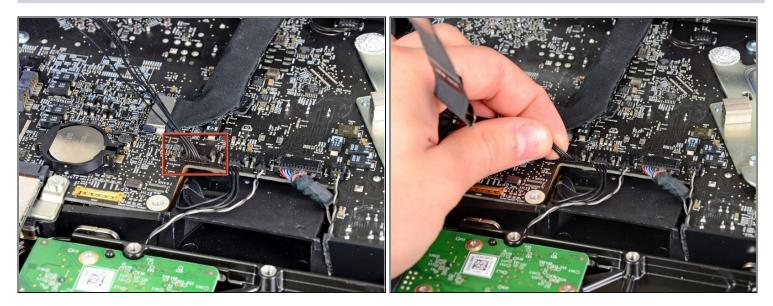
• Disconnect the LCD thermal sensor cable connector from its socket on the logic board.
