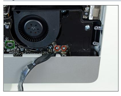
Remove two 5 mm T10 Torx screws securing the audio ports to the outer case.
