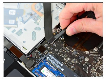
• Use the flat end of a spudger to pry the AirPort/Bluetooth connector up from its socket on the logic board.
