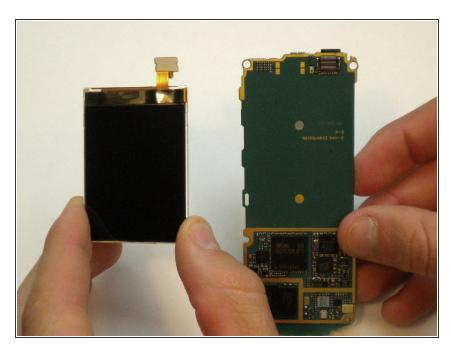
Unclip the ribbon plug located on the top of the LCD screen that connects it to the motherboard
