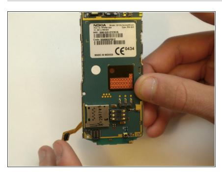
Unclip the faceplate plug (ribbon) located in the lower left corner of the motherboard
