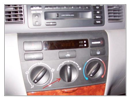
First, pry the trim up from around the shift lever, lifting straight up. Then, pull the fan speed knob out from the dashboard. Remove the screw from behind it.
