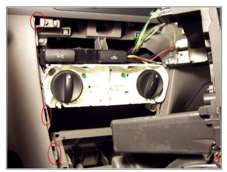
You'll need to carefully pull the whole instrument cluster out of the dashboard. The plastic clips circled in red are what is holding it in, so carefully pry there. A putty knife or other thin blade may help.
