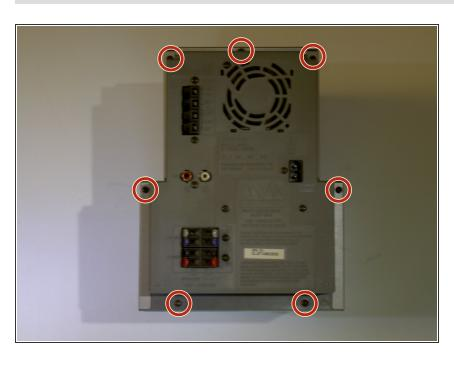
Remove these seven 11.5 mm screws and place aside.
