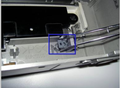
Using tweezers, remove the two restraints indicated and place with the screws removed in the previous step.
