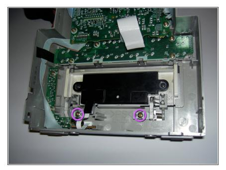
Remove the two 11.5 mm screws indicated and set aside in a safe place.
