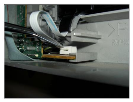
Using tweezers or fingers, pull firmly on the base of this cord until it pops out of its slot.
