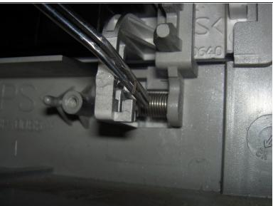
Remove the spring from its slot using tweezers.
