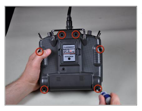
Remove the six screws around the back of the case.
