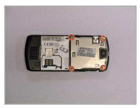
Using the T6 Torx Screwdriver, remove the four (4) T6 2mm Torx screws from the metal cover.
