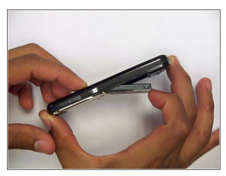
Remove the battery by pulling it away from the back of the phone.
