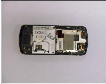
Remove the metal cover by inserting the flat end of the iFixit Opening Tool under the side of the cover, prying it away from the phone.
