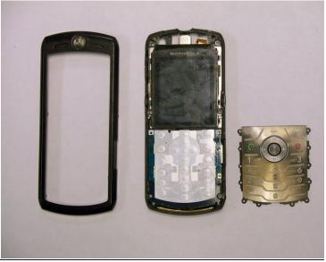
Remove the frame by inserting the flat end of the iFixit Opening Tool under the frame and prying it away from the phone.
