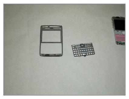
Once the front cover has been removed, there is nothing holding the keyboard to the rest of the phone. Simply remove the keyboard from the cover by lifting the keyboard from its interior side.
