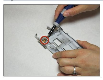
The volume control buttons are secured to the frame only by their fit around a small piece of the plastic. Using a small flathead screwdriver or other flat object, lift the ribbon over this piece of the cover.
