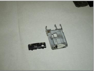
• After the logic board has been removed, there is nothing else securing the antenna to the back cover. Simply remove the antenna by pushing outward from the interior side.
