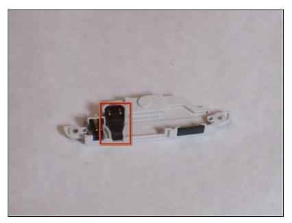
After the Connector Housing has been removed, there is nothing else holding the Microphone in place. Simply remove if from the housing by pulling up.
