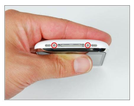
Remove the two 3.7mm Phillips #00 screws from the dock-connector end of the iPhone.
