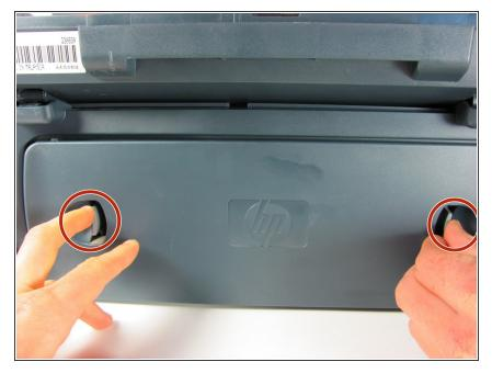
Remove the back panel by inserting your fingers into the indentations next to the tabs. Press the tabs inward towards each other while pulling the back panel toward you.
