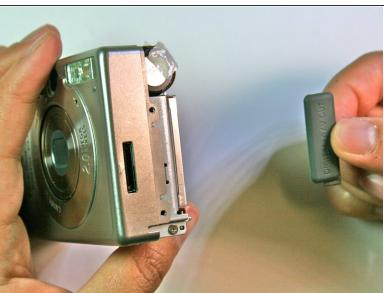
Slide the rubber digital a/v cap out of place on the front plate.
