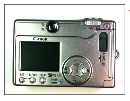
Remove the 3.8mm screw from the back face of the camera.
