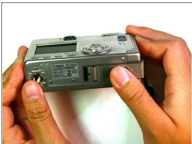
Slide the grey latch to open the battery compartment.
