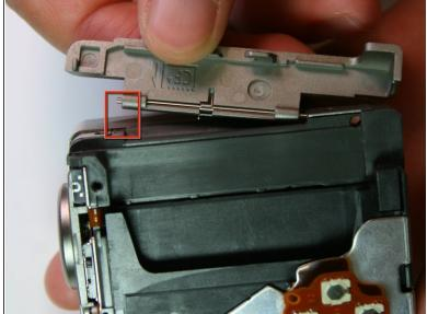
Remove the CF card door from the left side of the camera body.
