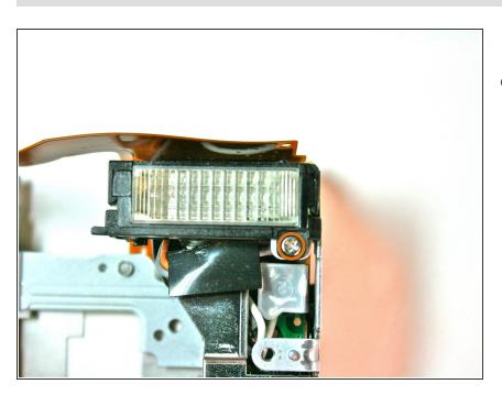
Remove the 3.3 mm screw from underneath the clear plastic flash unit on the front side.
