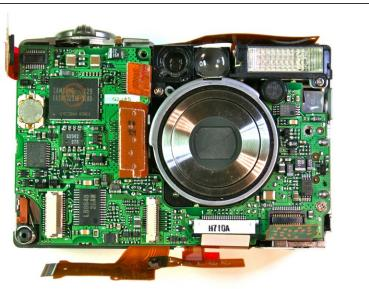
Remove the wire connections that connect along the bottom of the motherboard.
