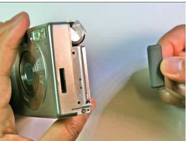
Slide the rubber digital a/v cap out of place on the front plate.
