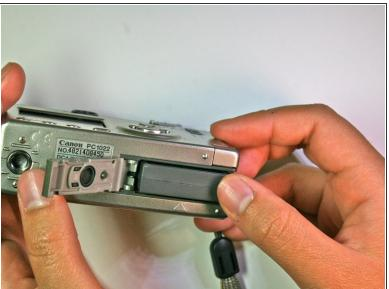
Push and slide the orange retaining clip to the right to remove the battery.
