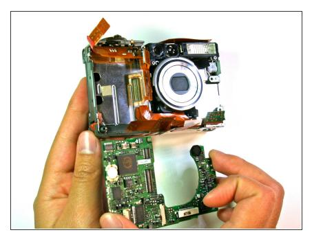
Remove the motherboard from the main frame of the camera body.
