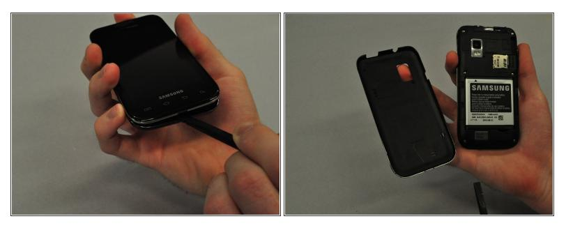
• Insert the edge of the spudger into the slit and use it to pry the back case off of the phone.
