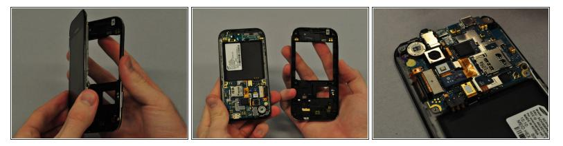
• Once the clips are detached, separate the main case from the LCD touchscreen.
