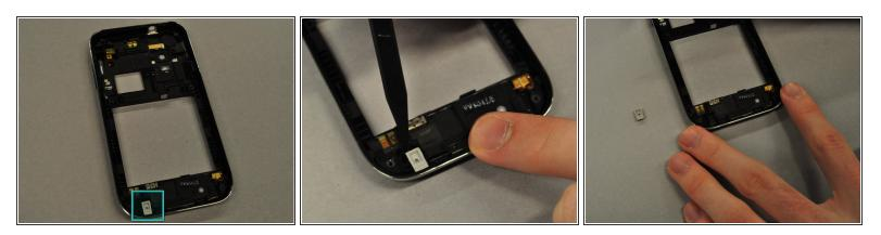
Use the spudger to pry out the grey rubber rectangular component from the main case.
