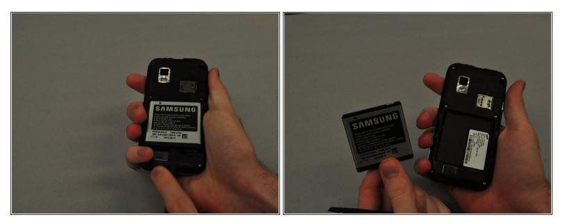
Insert the spudger into the space between the battery and the phone and pry the battery out as you slide it along the underside the battery.
